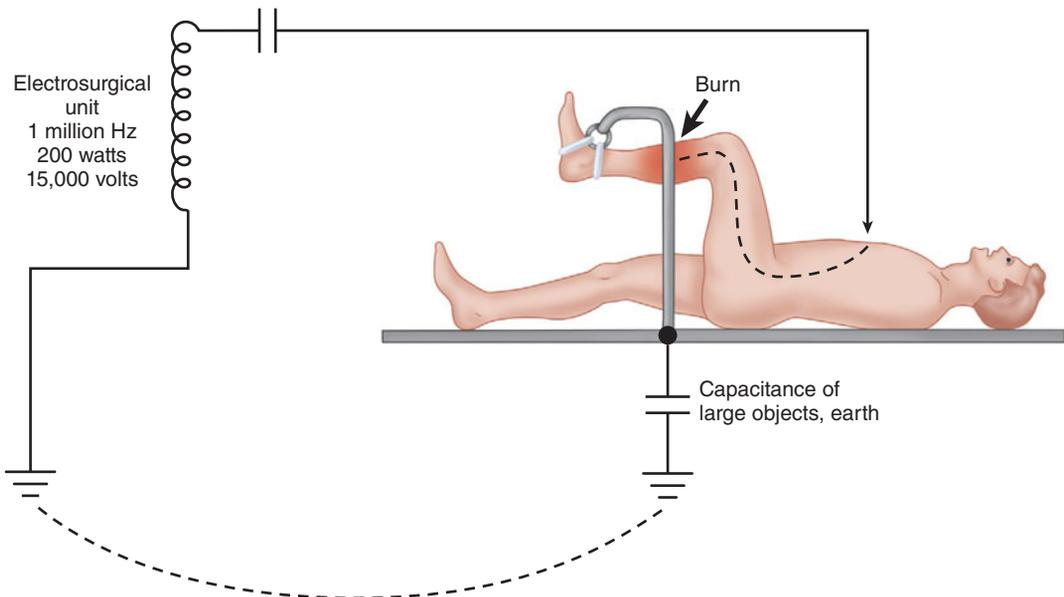
**FIGURE 2-10** Electro-surgical burn. If the intended path is compromised, the circuit may be completed through other routes. Because the current is of high frequency, recognized conductors are not essential; capacitances can complete gaps in the circuit. Current passing through the patient to a contact of small area may produce a burn. (A leg drape would not offer protection in the situation
