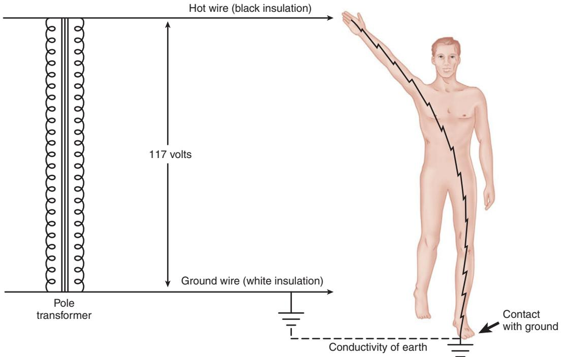
**FIGURE 2-6** The setting for the great majority of electric shocks. An accidentally grounded person simultaneously contacts the hot wire of the electric service, usually via defective equipment that provides a pathway linking the hot wire to an exposed conductive surface. The complete electrical loop originates with the secondary of the pole transformer (the voltage source)
