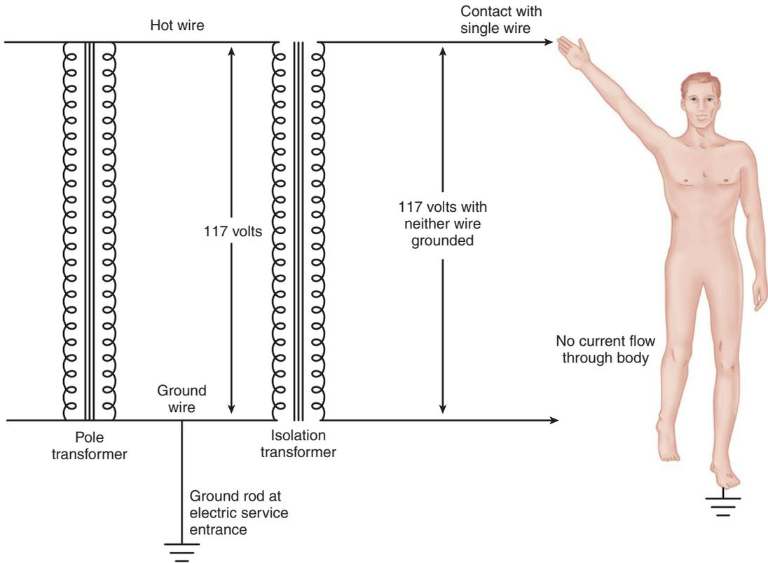
**FIGURE 2-8** Even though a person is grounded, no shock results from contact with one wire of an isolated circuit. The individual is in simultaneous contact with two separate voltage sources but does not close a loop
