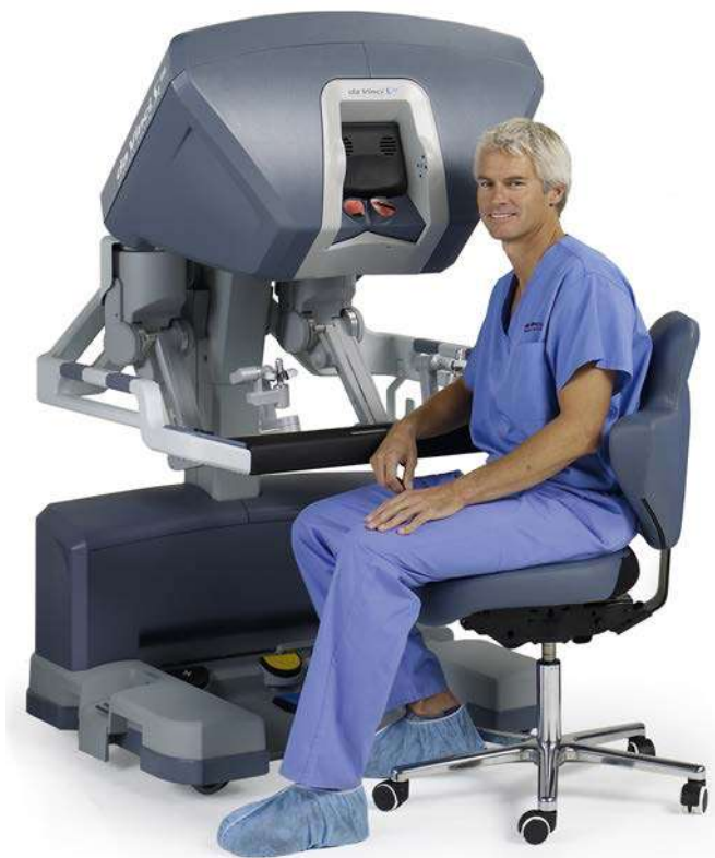
Fig. 71.4 The da Vinci Robotic Surgical System: the surgeon console. (Courtesy Intuitive Surgical, Sunnyvale, CA, USA)
