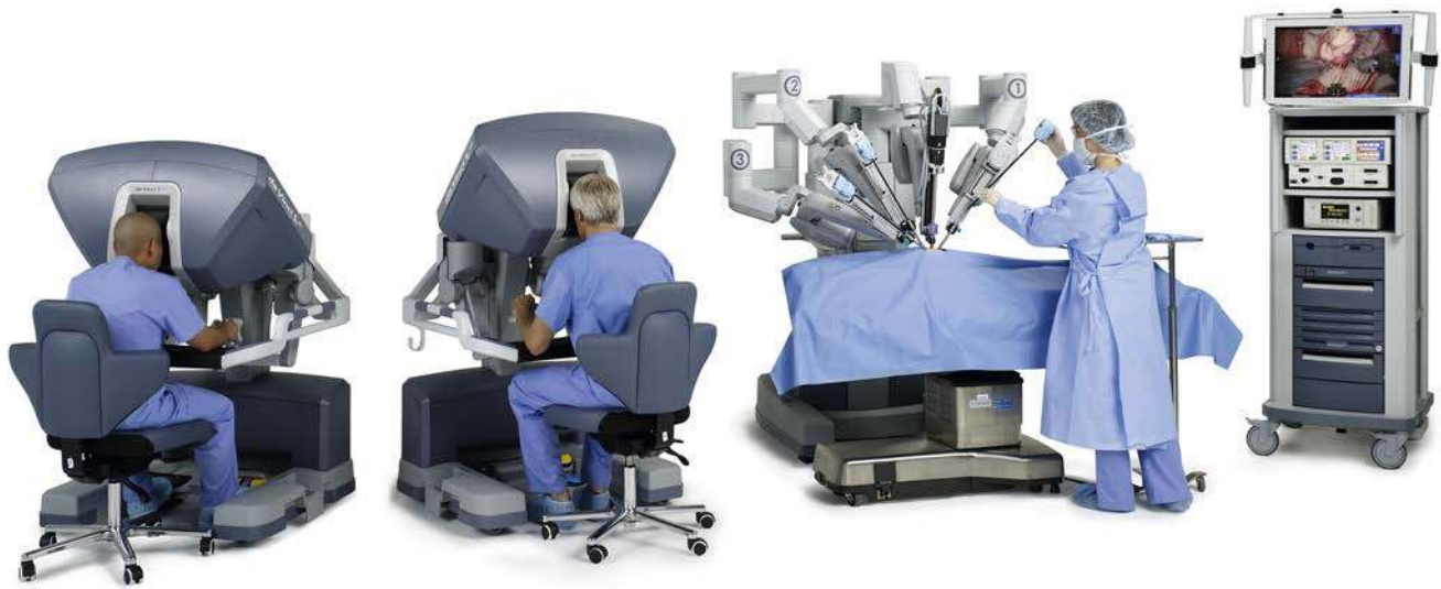
Fig. 71.2 The da Vinci Robotic Surgical System: two surgical consoles, patient-side cart with four mounted surgical arms, and an optical tower. (Courtesy Intuitive Surgical, Sunnyvale, CA, USA.)
