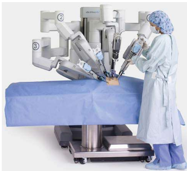
Fig. 71.9 The da Vinci Robotic Surgical System: patient-side cart. (Courtesy Intuitive Surgical, Sunnyvale, CA, USA.)
